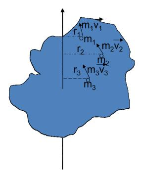
The angular velocities of all these point masses are same equal to  $\omega$  but linear velocities are different depending on their distance from the axis of rotation.
