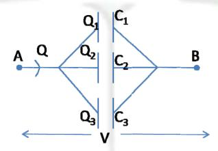
V= Potential difference between the points A and B. Since no potential difference takes place across a conducting wire hence potential of the first plate of all the three capacitors are same as that of A and potential of second plate of all the three are same as that of B. I.e. Potential difference across each of the three capacitors is V.
