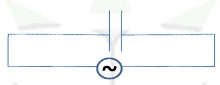
Let  $e = e_p \sin \omega t \rightarrow (1)$  be the applied emf at an instant of time t c = capacitance of the capacitor
