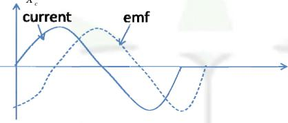
Comparing equation(1) & (4) we find that current through a capacitor leads the emf by a phase angle  $\pi/2$  or emf leads the current by phase angle  $\pi/2$
