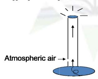
The velocity of the burning gas flowing through the burner being very high the pressure of the gas inside the tube is lesser than that of outside the tube. Hence air from outside rushes into the tube.
