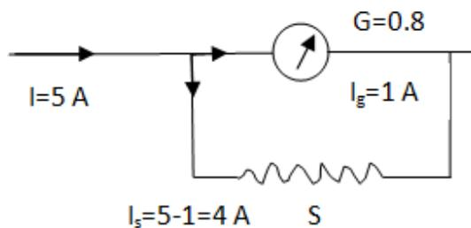
(i) To measure higher current shut resistance( $S$ ) to be connected in parallel to Ammeter.
