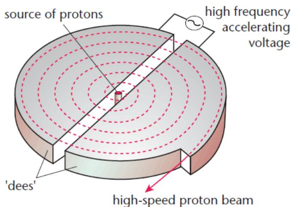
**Working:** A cyclotron consists of two D-shaped regions known as dees. In each dee there is a magnetic field perpendicular to the plane of the page. In the gap separating the dees there is a uniform electric field pointing from one dee to the other. When a charge is released from rest in the gap it is accelerated by the electric field and carried into one of the dees. The magnetic field in the Dee causes the charge to follow a half-circle that carries it back to the gap.
