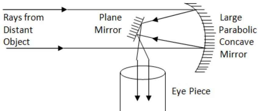
Advantage: Objective of reflecting telescope is a mirror (not lens), so the image formed is free from chromatic aberration (which occurs in lens as lens defect because of which image splits/spreads).
