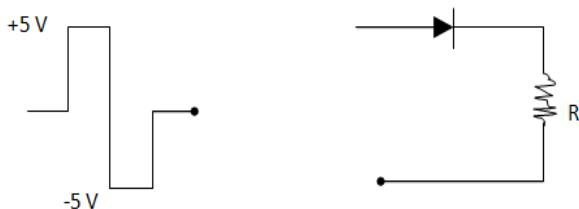
Answer: We know that diode gives output only when Anode (Collector) is at positive voltage and Plate (emitter) is at negative voltage, this we call as forward biased diode. In this given waveform when the input voltage is +5V, the diode gets forward biased, hence output across R is +5V will be obtained however during the next cycle of input waveform it clearly shows input voltage is -5V, the diode gets reversed biased so no output will be obtained across R.
