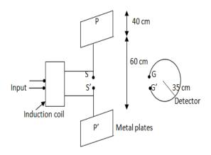
Experimental setup: Two large metal plates P and P' are connected to metal spheres S and S' as shown. The spheres are connected to an induction coil. High voltage is set-up across the gap by interrupting current in the coils. This voltage ionizes the air in the gap which produces oscillating current in the gap SS'.
