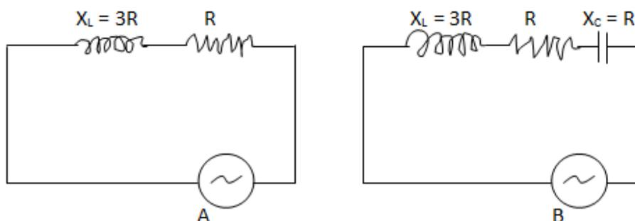
Calculate the ratio of power factor of the circuit B to the power factor of circuit A.
