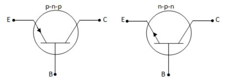
Thin and lightly doped base region contains very few majority charge carriers. This reduces the recombination rate of electrons and holes across the emitter-base junction. Also increases collector current and hence increases current gain of the transistor.
