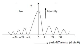
Width of central maximum: If d is the distance between slit and screen and y<sub>n</sub> is the distance of nth minimum from point O then
