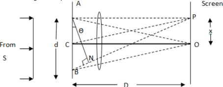
**Position of central maximum:** Let C be the center of the slit AB. According to Huygen's principle, when light falls on the slit, it becomes a source of secondary wavelets. All the wavelets originating from slit AB are in same phase. These secondary waves reinforce each other resulting the central maximum intensity at O.
