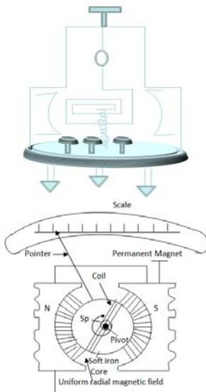
**Principle :** ( Based on the principle of the force of interaction between the current carrying conductor and a magnetic field) A coil is suspended in a magnetic field. The current to be measured is passed through the coil. The current through the coil produces a magnetic field which interacts with the given magnetic field in which the coil is suspended. Due to the interaction the coil gets deflected and measuring the angle of rotation current can be calculated.
