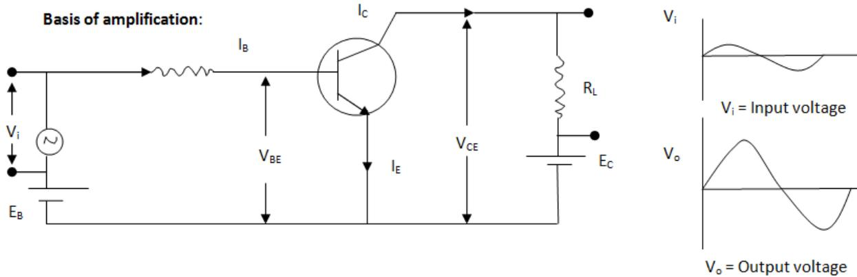
Above circuit shows n-p-n transistor in common emitter mode. The battery  $E_B$  provides biasing voltage for base-emitter junction.  $V_{CE}$  voltage between collector and emitter maintained by using battery  $E_C$ .
