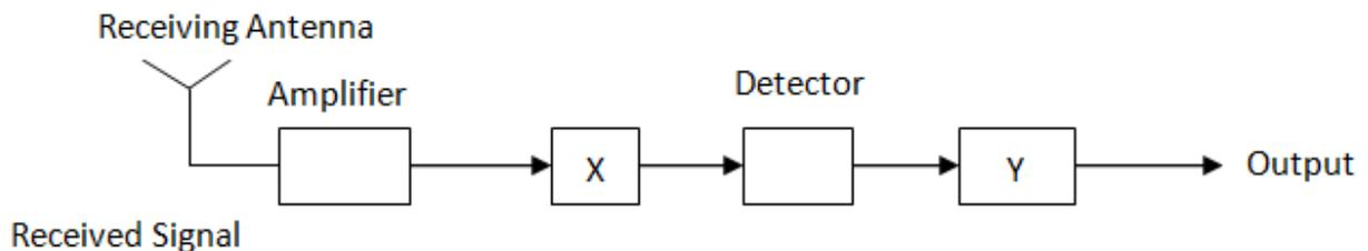
**Answer:** X is Intermediate Frequency (IF Stage) stage; here the received signal for antenna is converted to lower frequency signal call Intermediate Frequency.
