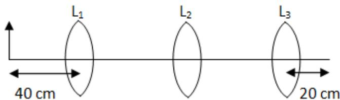
**Answer:** Considering the first lens  $L_1$ , focal length = 20 cm,  $u = 40$  cm, it means object PQ is kept at  $2f$  from convex lens  $L_1$  hence image  $P'Q'$  will be formed at  $2f$  i.e. 40 cm on the other side of  $L_1$ .
