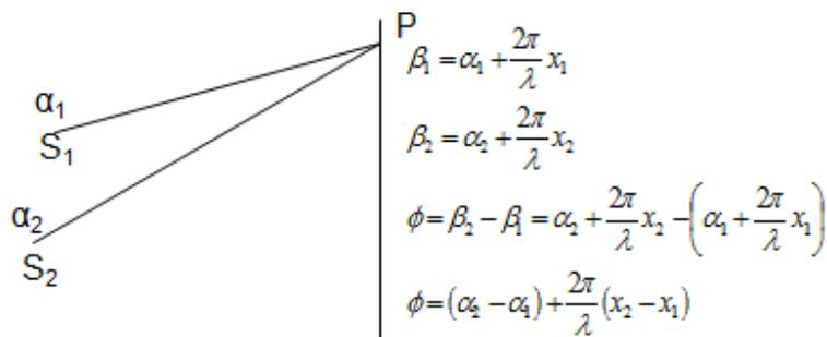
Let  $y_1$  and  $y_2$  be the displacement at any point  $P$  on the screen at an instant of time  $t$  of the waves emitted from  $S_1$  and  $S_2$  respectively. Using displacement equation:
