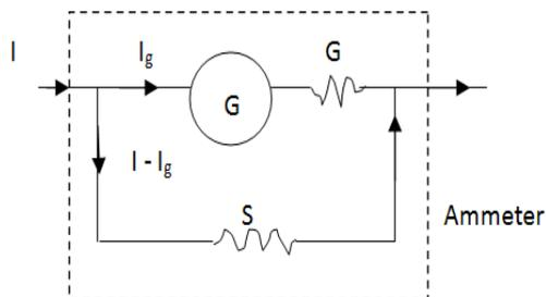
Let  $I_g$  be the current with which the galvanometer gives full scale deflection. Since galvanometer and shunt are connected in parallel then
