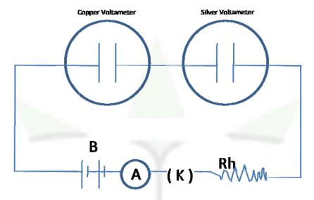
The electrodes which acts as cathode from both the voltameters are taken out cleaned dried and weighed and are again placed in their position. Closing the key K a constant current is passed through the series circuit for a given time interval. The electrodes at the cathode are taken out dried and weighed and then the mass of ions deposited are calculated.
