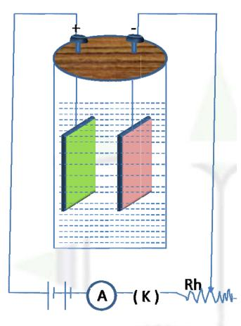
A copper voltammeter is taken and by trial rheostat is adjusted so that suitable constant current flows through the circuit as shown. The copper plate connected to the negative terminal i.e. the plate acting as cathode is thoroughly cleaned dried and weighed and then again placed in its position.
