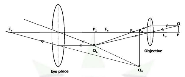
It consists of objective and eye piece. The objective is a convex lens of small aperture and small focal length. The aperture of the eye piece lens is slightly greater and the focal length is also small.
