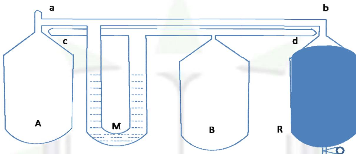
The thermometric part consists of a bulb of silica A connected to an exactly similar bulb R through a capillary tube ab, bent twice at right angles. A is known as the bulb of the thermometer and R is filled with mercury by opening the outlet the mercury can be taken out from the bulb.
