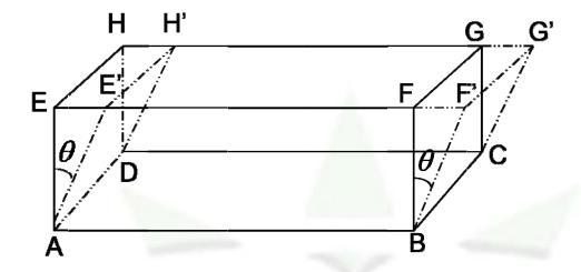
The applied force f per unit area of the surface to which the force is parallel is known as shearing stress or tangential stress = F/a
