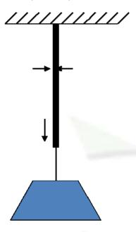
L & D = original length and diameter of the wire.
