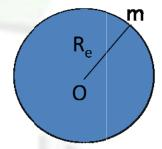
F = Weight of the particle. This force towards the center of earth produces acceleration towards the center of earth and since this acceleration is produced by the gravitational force it is known as acceleration due to gravity & is represented by g
