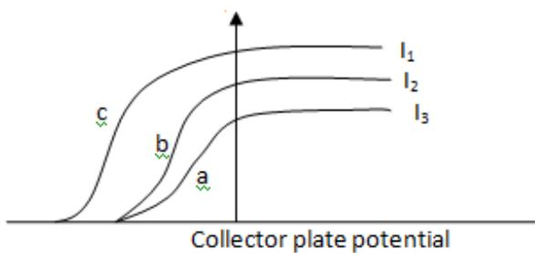
The stopping potential  $V_s$  is same for a and b, hence frequencies of incident light are same for a and b curve, but intensities are different ( $I_2 > I_1$ ).
