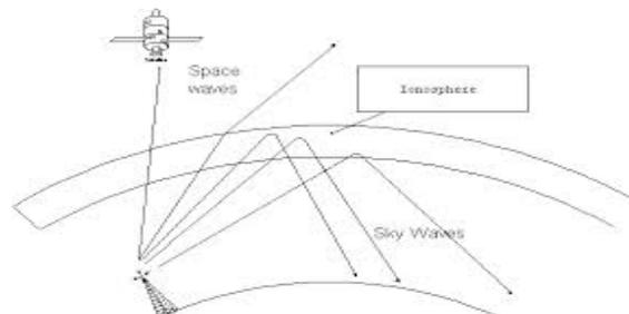
Radio waves from the transmitting antenna reach the receiving antenna after reflection in the ionosphere, this wave propagation is called *sky wave propagation*.
