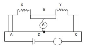
The figure shows experimental set up of a meter bridge. When the two unknown resistances X and Y are inserted, the null point D is obtained 40 cm from the end A. when the resistance of  $10~\Omega$  is connected in series with X, the null points shifts by 10 cm. Find the position of the null point when the  $10~\Omega$  resistance is instead connected in series with resistance 'Y'. Determine the values of the resistances X and Y.
