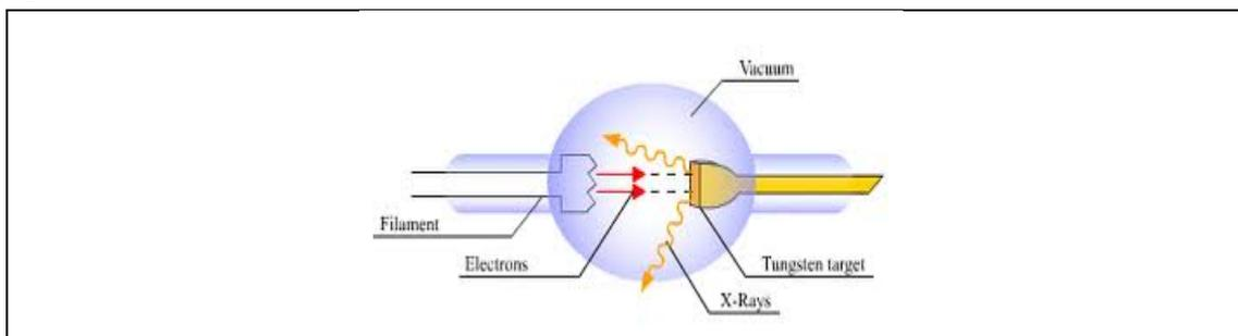
X-ray: How it emits, actually high speed electron when enters to the electric field of electrons its velocity decreased, energy decreased, decreased energy comes out in the form of radiation ( X-ray), once struck the orbital electrons of target, hit electrons go to higher level, electron jumps from higher level and difference of energy emitted in the form of X-ray (more you will read when time will come).
