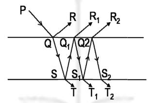
If we consider any two members in a particular series say QR and  $Q_1R_1$  since they are obtained from the single ray PQ hence they are coherent and produces interference fringes where reunite. This is cause of colour of thin film.
