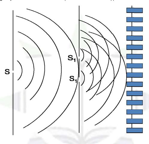
S1S2 = distance between the pin holes on the second board. It is small of the order of millimeter. On the screen we get alternative bright and dark fringes.
