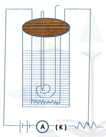
A copper calorimeter is taken and about 2/3<sup>rd</sup> of the calorimeter is filled with water and a thermometer is inserted into the water in the calorimeter. A resistance coil is immersed into the water in the calorimeter and the two ends of the coil are connected to two terminal screws at the top of the box in which the calorimeter is kept. A battery B an ammeter A, a key and a rheostat connected in series with the two screws.
