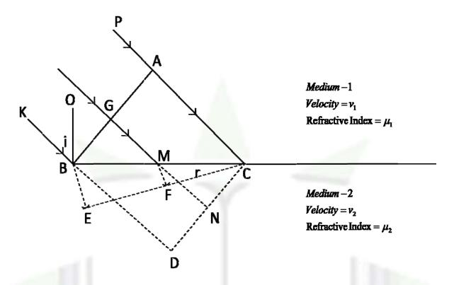
BC is the section of the refracting surface by the plane of the paper i.e. the out face, separating two media of refractive indices  $\mu_1$  and  $\mu_2$  ( $\mu_1 < \mu_2$ )
