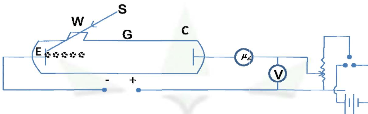
G is a glass discharge tube having a window W of quartz which allow the ultraviolet light to pass through. E is the emitting surface and C is the collecting electrode. A potential difference known as accelerating potential difference is applied between the two electrodes by using a potential divider arrangement and commutator and the applied potential difference is measured by a voltmeter. The photo electric current flowing in the circuit is measured by micro ammeter.
