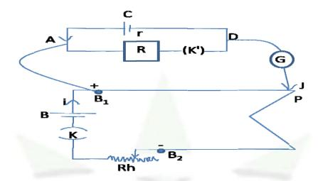
(1) Key K<sup>'</sup> is kept open no current flows through R i.e. The circuit of the test cell is an open circuit. The balance point is found by using the test cell C.
