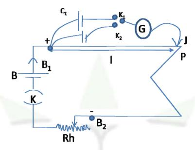
If K1 is closed (  $K_2$  is open ) balance point is found by using  $C_1$
