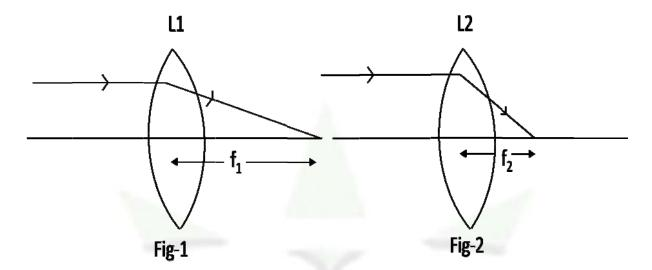
Comparing the two figures, we see that the converging power of lens L2 is greater than that of lens L1, but focal length of lens L2 is smaller than that of lens L1. Hence we conclude that the power & focal length of a lens are inversely related i.e. when one is greater than other is smaller.
