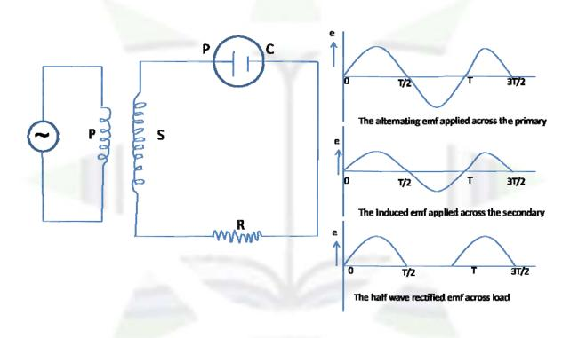
During the first half cycle the induced emf makes the plate of the valve at (+)ve potential with respect to the cathode hence the valve conducts current in the circuit. This current being varying the potential difference V= iR across the resistance also varies exactly in the same way.
