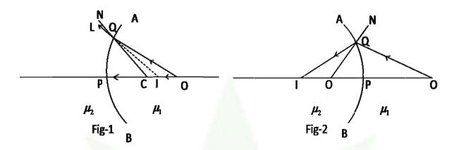
AB is a spherically curved surface, separating the two media of refractive indices &  $\mu_2$  ( $\mu_2 > \mu_1$ ). In figure-1 the concave surface faces the rarer medium & in figure-2  $\mu_1$  the convex surface faces the rarer medium. A point object O is taken in the rarer medium on the principal axis.
