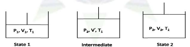
In passing from state 1 to state 2 let us consider an intermediate state which is obtained as follows, temperature is kept constant at  $T_1$ , pressure is changed from  $P_1$  to  $P_2$  and let the volume change from  $V_1$  to  $V^{'}$
