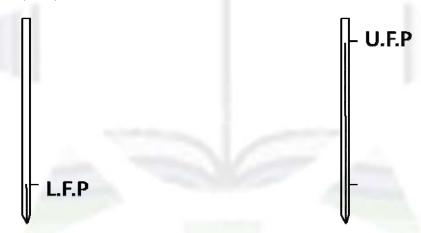
**Upper Fixed Point** (U.F.P): The bulb of the thermometer is immersed in boiling water in a hypsometer where water is boiled at normal pressure. The level up to which Hg rises in the capillary tube is marked and is known as upper fixed point. It is 100°C or 212°F or 80°R.
