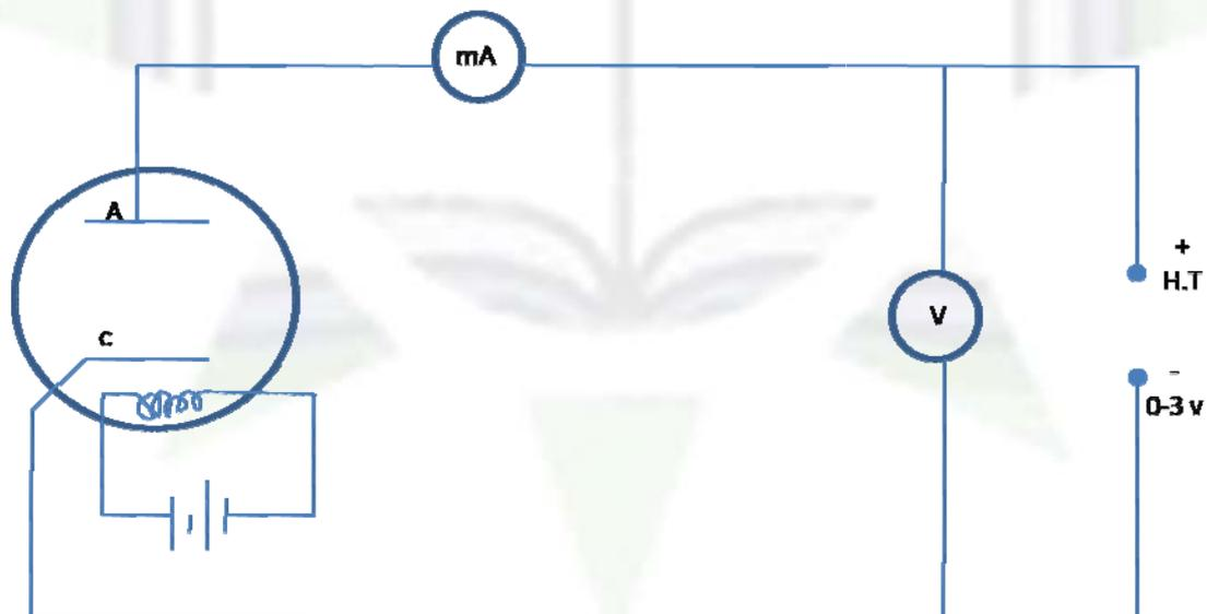
**Action of diode:** On heating the filament the cathode is heated and the electrons are emitted. In order to collect the electrons by the plate the plate is to be kept at (+) ve potential with respect to the cathode. The electrons flow through the plate circuit giving plate current  $i_p$  or anode current  $i_a$ . The current is in millie ampere range and is measured by the millimetre.
