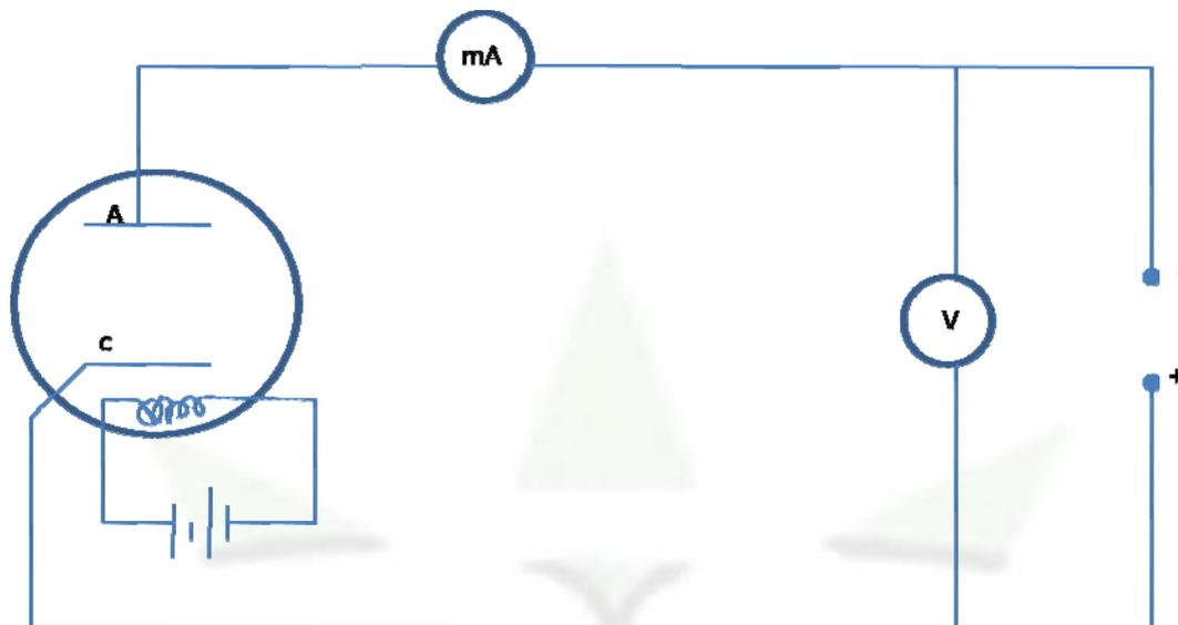
When the plate is kept at negative potential with respect to the cathode no plate current flows through the circuit electrons emitted from the cathode will not be attracted by the plate and hence no electron will be able to reach the plate, the plate current becomes zero. Thus diode allows current to flow in one direction only and due to this uni-directional flow it is known as valve.
