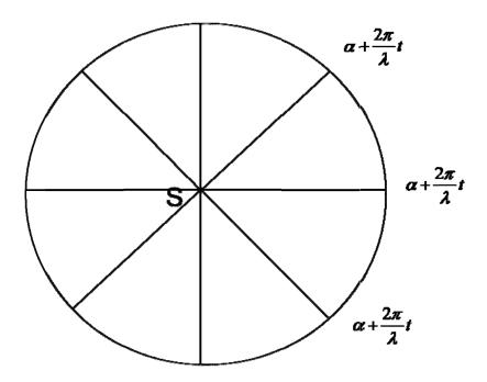
Let S be a point source of light. To find the points where the light from source S will reach after a time t with S as center and c x t as radius we imagine a sphere this imaginary sphere is known as the wave front an instant of time t.
