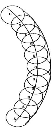
Since every point on the surface of a wave front acts as a secondary source of light hence every points emits a spherical wave front. The imaginary plane in the forward direction which can be drawn by touching the entire sphere which is emitted at the same time is the position of the wave front at that time.
