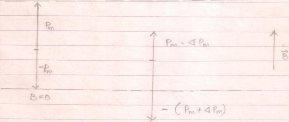
When no magnetic field is applied the orbital magnetic moment of the two electrons being equal and opposite will mutually cancel out. But in the presence of the external magnetic field  $\vec{B}$  the magnetic moment in a direction of the field decreases while that in opposite direction increases.
