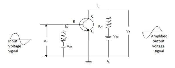
The input (base-emitter) circuit is forward biased and the output (Collector-emitter) circuit is reversed biased.
