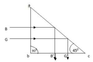
$\mu=A+\frac{B}{\lambda^2}$ , we know wave length of Red (R) is maximum; hence refractive index of this prism for red will be minimum. Also we have  $\mu_1 sini=\mu_2 sinr$ , and critical angle for red is maximum hence except red colour Green and Blue light rays will incident at ac surface more than the critical angle hence blue and green will suffer total internal reflection where as Red will emerge out for ac face.
