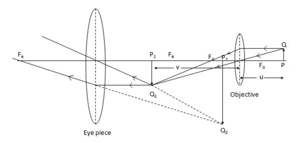
**Ray diagram**: PQ is an object kept in front of objective ( $f_0 < u < 2 f_0$ ),  $P_1Q_1$  is the image formed by objective this image serves as object for eye piece, since  $P_1Q_1$  lies between the focus and optical center of eye piece hence an extended image  $P_2Q_2$  is formed by eye piece. Thus  $P_2Q_2$  is the final image of PQ produced by the compound microscope.
